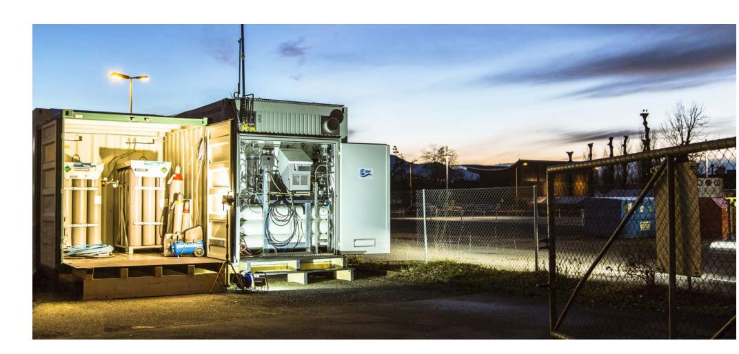
Figure 3: Demonstration plant for production of renewable methane in Rapperswil.
