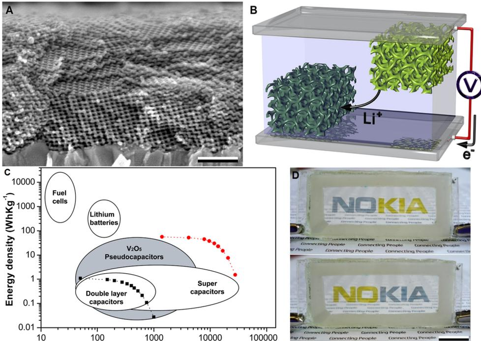
Nanostructuring electrode materials at the 10nm length scale increases the performance of batteries and supercapacitors.
