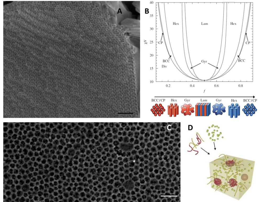
Sol-gel chemistry affords the synthesis of various metal oxides and can be directed by block-copolymer self-assembly. The precursor sol complexes with one of the polymer blocks and is compartmentalised by the self-assembly process that sets in during solvent evaporation, leading to a 10nm pore-structure (scale bars: 200 nm).
